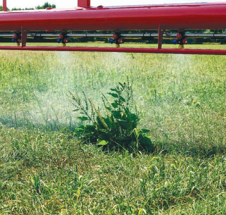
Bilberry's green-on-green solution harnesses artificial intelligence, which uses algorithms that detect and spray weeds in real time. Photo: Josh Johnson
