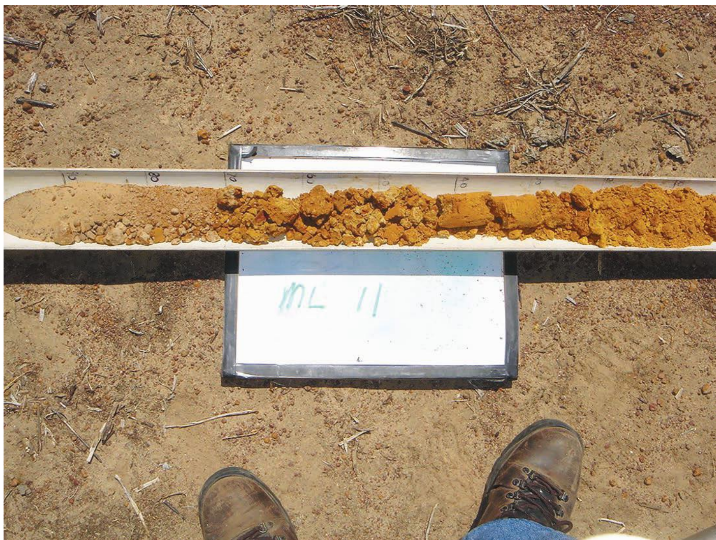
With agronomist Luke Marquis, Mic Fels and his team deep soil cored and tested representative sites chosen from key zones found on the EM38 maps.
