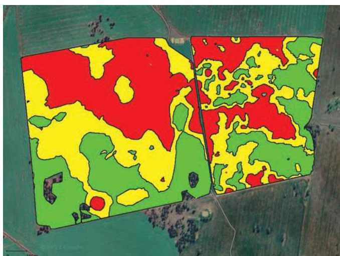
Figure 5.13: Three soil zones developed from the EM map of Burrungong and Oaks paddocks.
