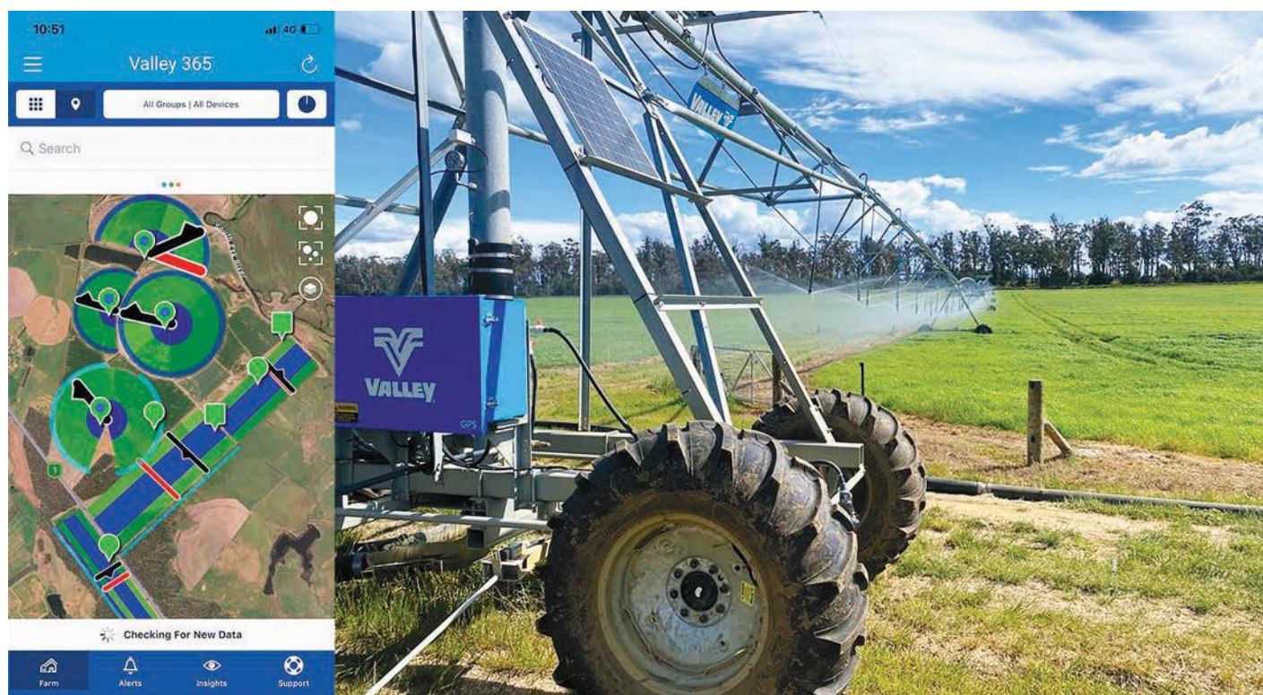
All of the Tait's lateral move irrigation systems are running with GPS guidance using app-based controls.
