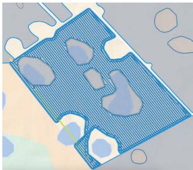
Figure 8.5: SwarmFarm path plan.
