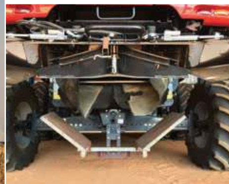
ABOVE: Harvesters can easily be equipped to produce narrow windrows. LEFT: Narrow windrow burning is a low-cost, highly-effective non-chemical weed control option in low-rainfall areas. Photos: Ben White
