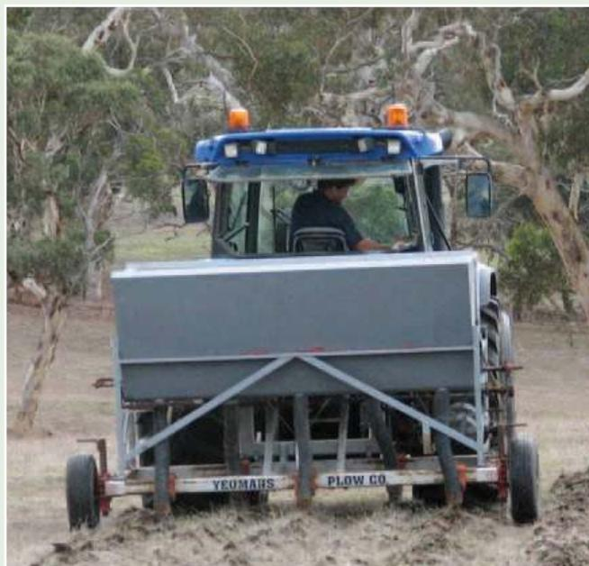
**Figure 5: Incorporation of lime using Yeoman's plough**
